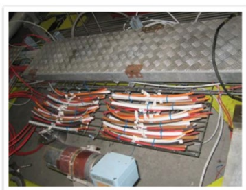
Fig. 1 – Cable witnesses exposed in real conditions of use (CERN- LHC)
