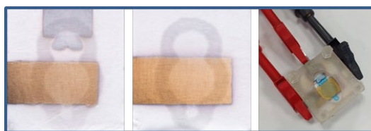
Figure 1. Photographs of a microfluidic electrochemical cell obtained by integrating EPF electrodes with chromatographic paper.
