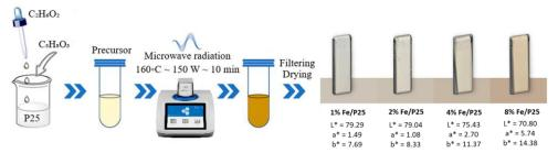
Figure 2. Microwave-assisted synthesis of Fe(III) oxides-TiO<sub>2</sub> (P25) heterojunctions and visual appearance of coatings at varying iron (III) amounts
