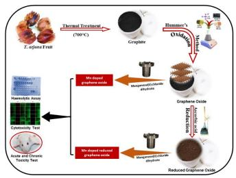
Figure 1. Optimal Manganese-doped GO and rGO synthesised from dried T. arjuna fruit
