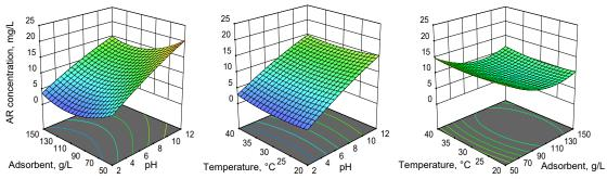
Figure 1. RSM 3D representations of the effect of pH, adsorbent dose and temperature on the final concentration of Acid red 66
