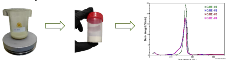
Figure 1. The combination of nanocellulose and basil extract; DTG diagram of NC/BE systems
