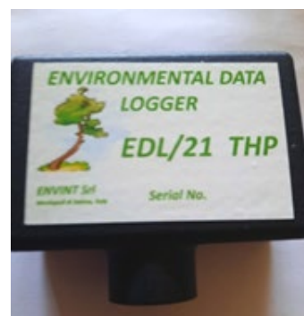
Figure 1. (A) Analyst assembling and (B) typical movable Datalogger for the thermo-hygrometric parameters recording.
